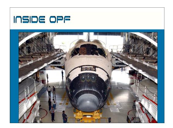
At the OPF, the orbiter is prepared for it's next flight. Panels fold down all around the orbiter at the OPF to allow personnel to access the different locations on the orbiter. The Payload may be installed horizontally at the OPF or vertically at the launch pad.
