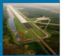
The SLF runway was made specifically for Orbiter landings. The runway is about 3 miles long, and has 1000' overruns on each end. It's also 300' wide (length of a football field), and is sloped for drainage purposes.
